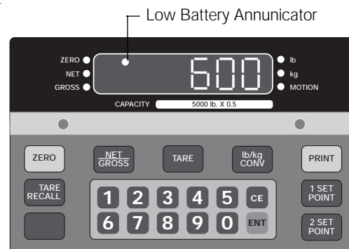
Figure 2-2. Low Battery LED Annunciator
